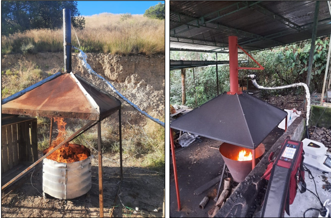
Supplementary Figure 1: Illustration of the small (left) and mid-size (right) metal Kon-Tiki with the hood and chimney for emission assessment.
