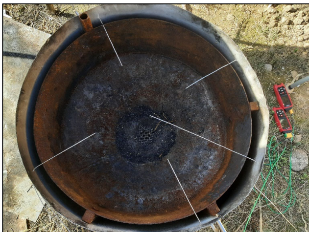
Supplementary Figure 4 : Installation and distribution of the Type K thermocouples in the Kon-Tiki kiln.
