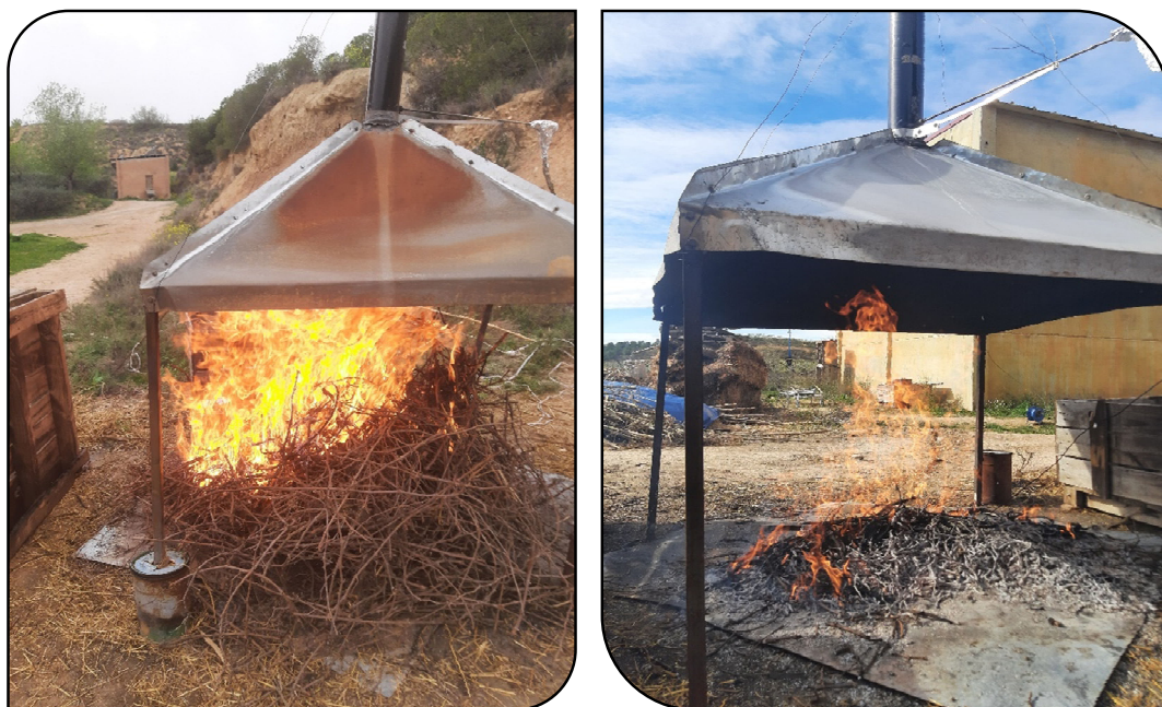
Supplementary Figure 2: Illustration of the open burning events of pile-up biomass under the hood and chimney for waste gas analysis.
