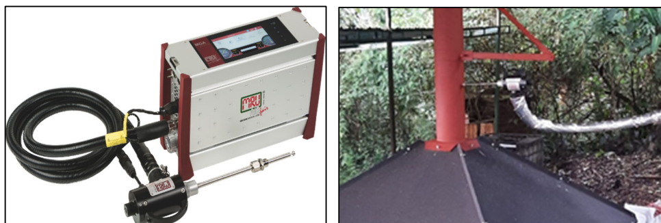
Supplementary Figure 3: MRU MGAprime flue gas measurement analyzer with probe (left) and installation of the gas measurement probe in the flue gas stream (right). Picture source: https://www.mru.eu/produkte/detail/mgaprime-q/
