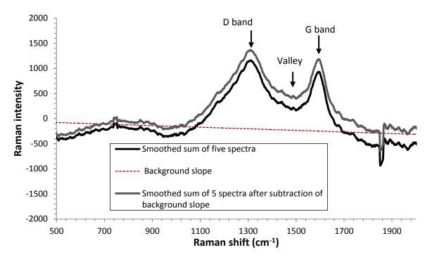
Figure 1: Spectra based on sum of five sub-samples showing subtraction of photoluminescence slope for the Cone kiln sample.
