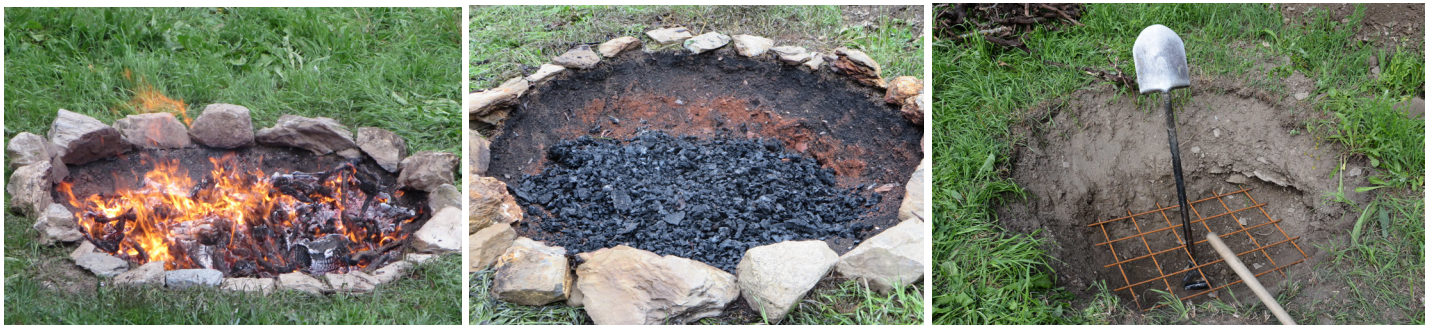
Fig. 6: Production of biochar in a 90 cm deep pit with a stone rim (Images: Ithaka-Institute).
